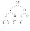
(b) The first 5 insertions produce the tree  $T_1$  with no rotations. The next insertion of key 2 produces  $T_2$  which is double-rotated into  $T_3$ . Inserting key 7 causes a rotation to produce  $T_4$ . Inserting keys 6 and 4 causes no rotation, yielding  $T_5$ . Finally, deleting 9 from  $T_5$  causes a rotation, yielding  $T_6$ .
