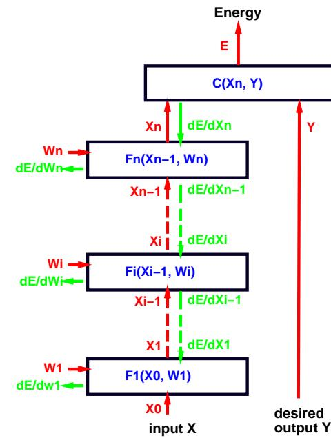
$$\frac{\partial E}{\partial X_{i-1}} = \frac{\partial E}{\partial X_i} \frac{\partial F_i(X_{i-1}, W_i)}{\partial X_{i-1}}$$
