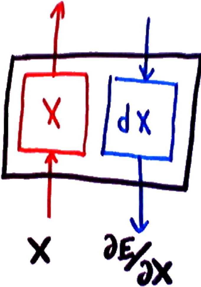
the internal state of the network will be kept in a “state” class that contains two scalars, vectors, or matrices: (1) the state proper, (2) the derivative of the energy with respect to that state.
