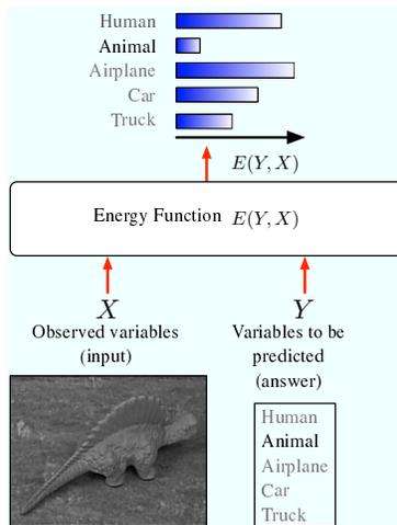
Figure 1: A model measures the compatibility between observed variables  $X$  and variables to be predicted  $Y$  using an energy function  $E(Y, X)$ . For example,  $X$  could be the pixels of an image, and  $Y$  a discrete label describing the object in the image. Given  $X$ , the model produces the answer  $Y$  that minimizes the energy  $E$ .
