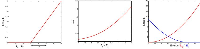
Figure 5: The hinge loss (left) and log loss (center) penalize  $E(W, Y^i, X^i) - E(W, \bar{Y}^i, X^i)$  linearly and logarithmically, respectively. The square-square loss (right) separately penalizes large values of  $E(W, Y^i, X^i)$  (solid line) and small values of  $E(W, \bar{Y}^i, X^i)$  (dashed line) quadratically.
