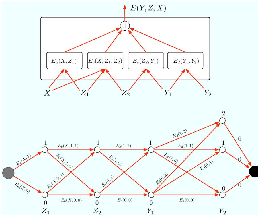
Figure 19: *Top: A log domain factor graph. The energy is a sum of factors that take different subsets of variables as inputs. Bottom: Each possible configuration of  $Z$  and  $Y$  can be represented by a path in a trellis. Here  $Z_1$ ,  $Z_2$ , and  $Y_1$  are binary variables, while  $Y_2$  is ternary.*
