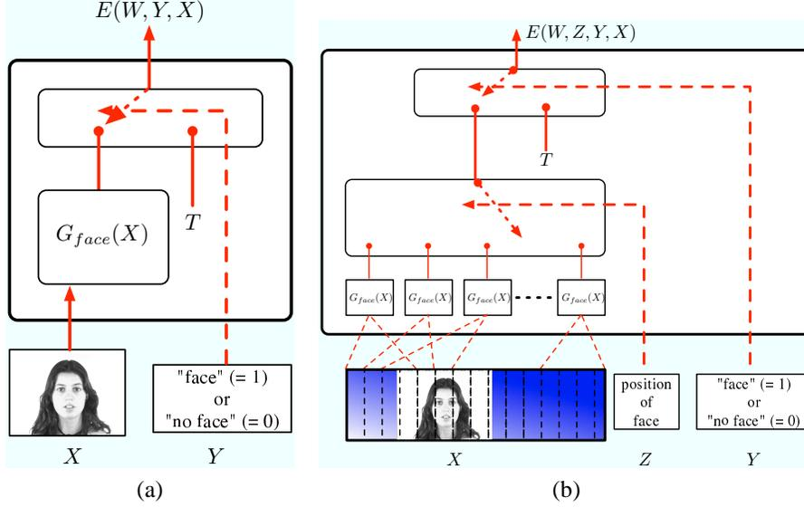
Figure 8: (a): Architecture of an energy-based face detector. Given an image, it outputs a small value when the image is filled with a human face, and a high value equal to the threshold  $T$  when there is no face in the image. (b): Architecture of an energy-based face detector that simultaneously locates and detects a face in an input image by using the location of the face as a latent variable.
