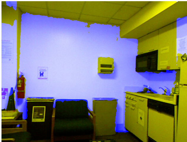
Figure 5. A demonstration of our scheme for finding the boundaries of the room. In this scene, the blue channel has been replaced by a binary mask, set to 1 if the depth of point is within 4% of the maximum depth within each column (and 0 otherwise). The walls of the room are cleanly identified, while segmenting objects of similar depth such as the fire extinguisher and towel dispenser. On the right, the cabinets and sink are correctly resolved as being in the room interior, rather on the boundary.
