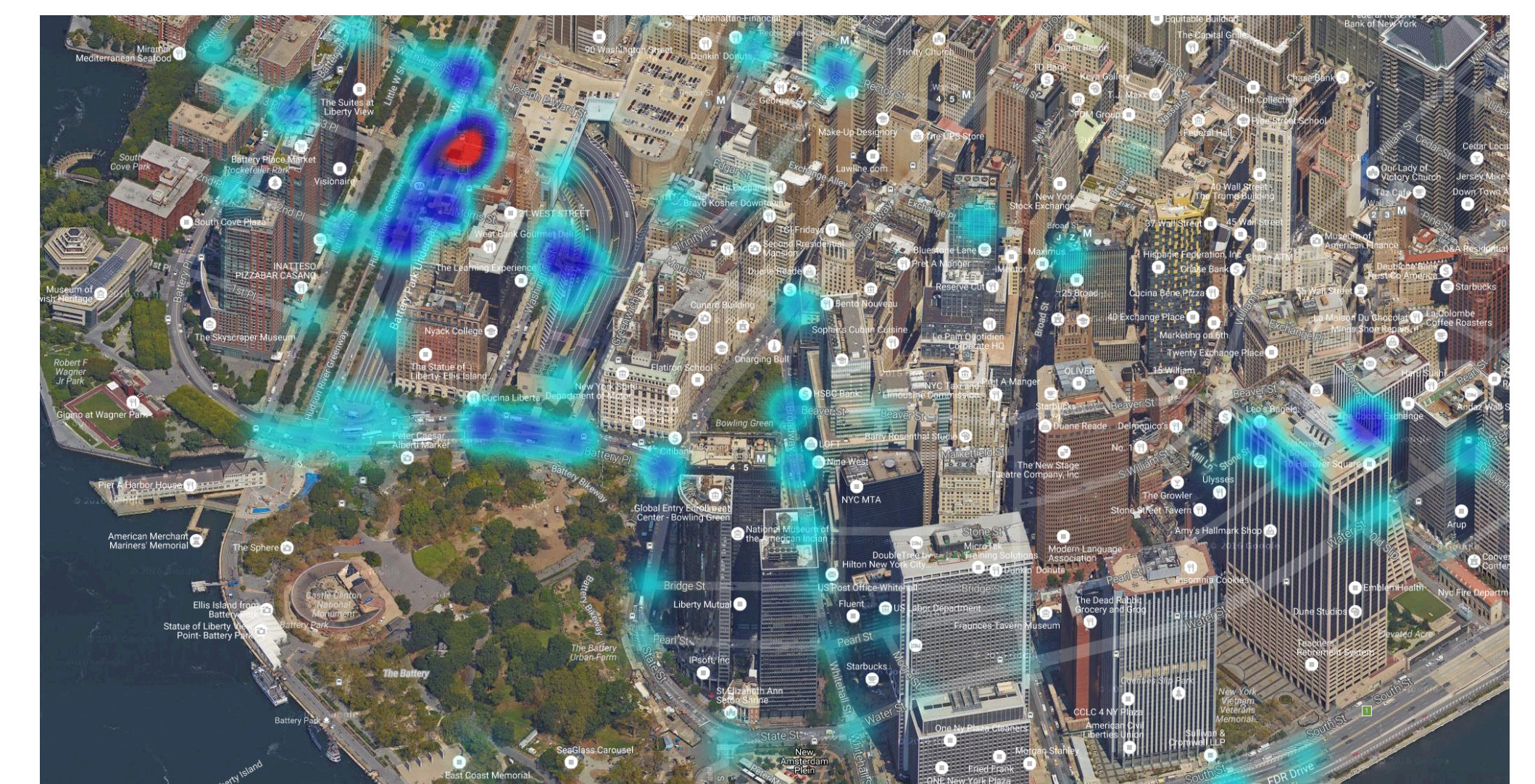
Figure 4: Heatmap of significantly increased wind velocity at pedestrian level from 1999 to 2016 at Lower Manhattan.
