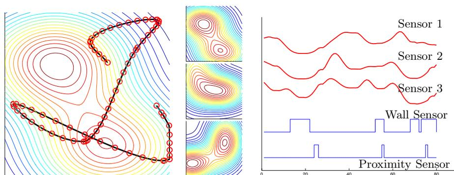
**Fig. 1.** Typical noisy sensor readings seen by a single agent. The first three sensors are continuous valued sensors; the fourth is a wall-detecting binary sensor. The proximity sensor indicates whether an agent is in the close proximity with other agents.
