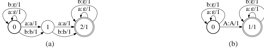
Fig. 2. Count-based kernels for the alphabet \Sigma = \{a, b\} . (a) Bigram kernel transducer. (b) General count-based kernel transducer.
