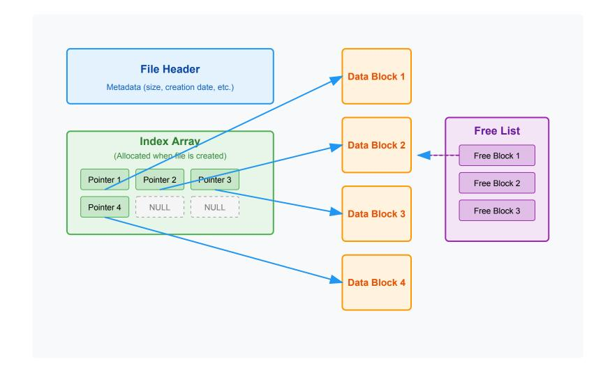
Each file has an array containing pointers to all its data blocks
