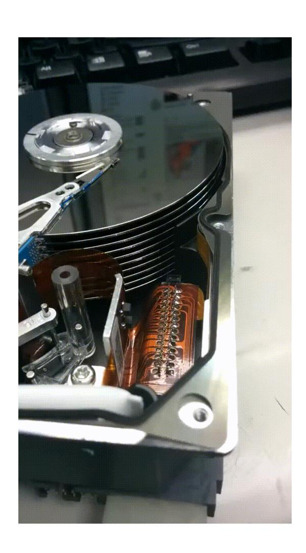
Rotate together on central spindle (3600-15000 RPM)
