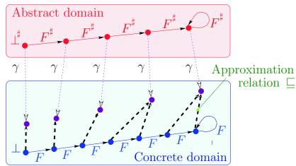
$$F \circ \gamma \sqsubseteq \gamma \circ F^{\sharp} \Rightarrow \operatorname{lfp} F \sqsubseteq \gamma(\operatorname{lfp} F^{\sharp})$$
