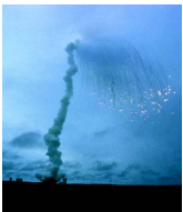
Ariane 5.01 failure (overflow)
