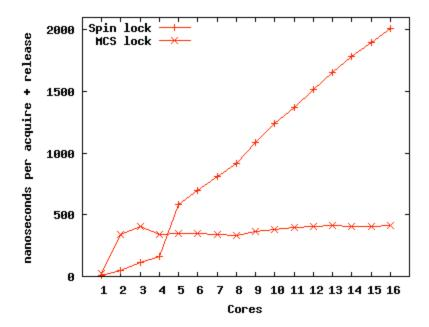
Time required to acquire and release a lock on a 16-core AMD machine when varying number of cores contend for the lock. The two lines show Linux kernel spin locks and MCS locks (on Corey). A spin lock with one core takes about 11 nanoseconds; an MCS lock about 26 nanoseconds.
