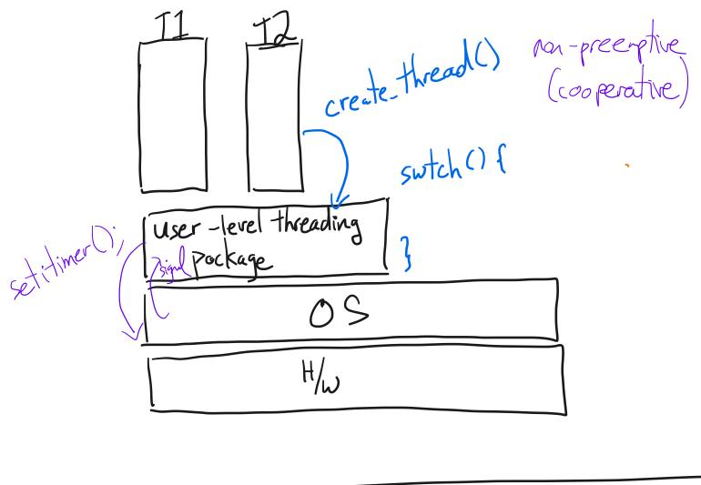
4. Context switches (user space) T3 stack - switch registers active Eswitch page tables MI stack TZ stack
