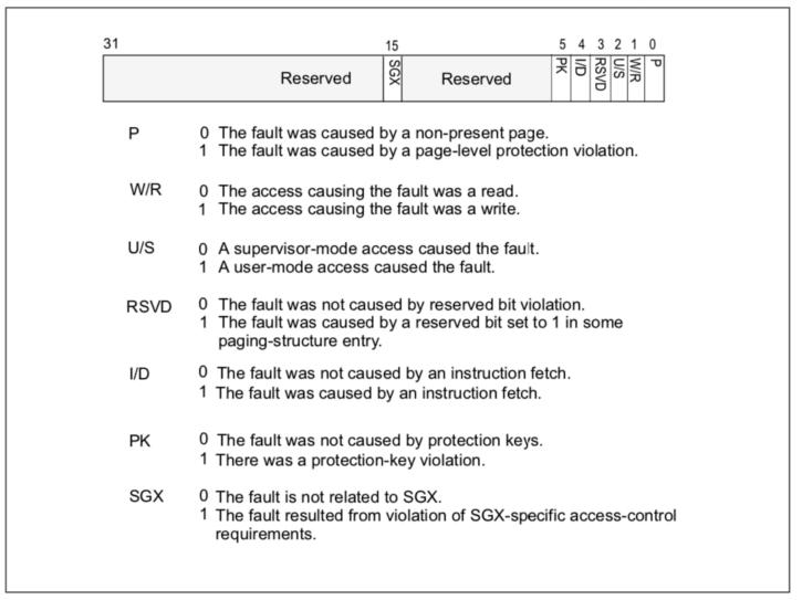
Figure 4-12. Page-Fault Error Code
