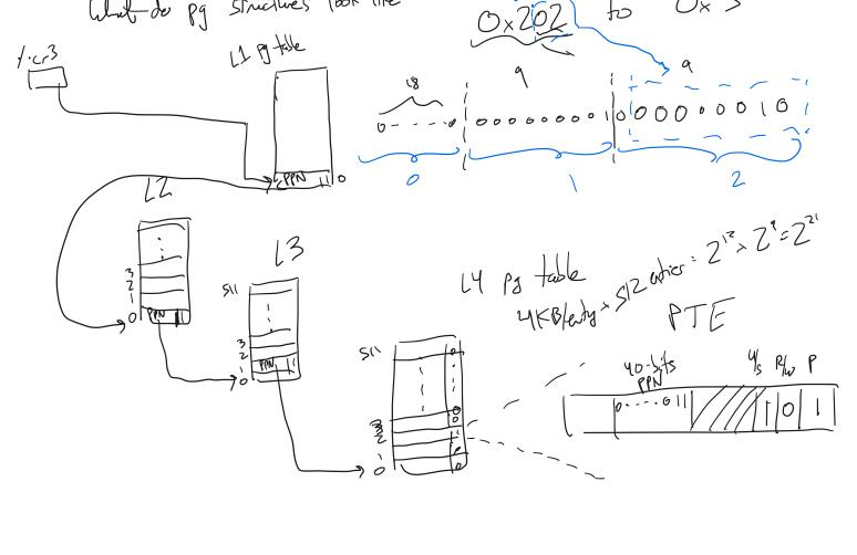
VPN, 4PPN, Perms x 86, ARM MIPS TLB miss ? Pg fault (No!) Pg fault ? TLB miss (No!) enty cold be Read-only
