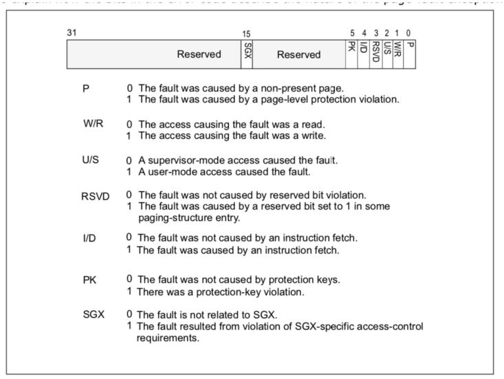
Figure 4-12. Page-Fault Error Code
