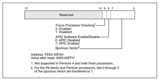
Figure 8-23. Spurious-Interrupt Vector Register (SVR)
