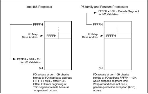
Figure 17-1. I/O Map Base Address Differences
