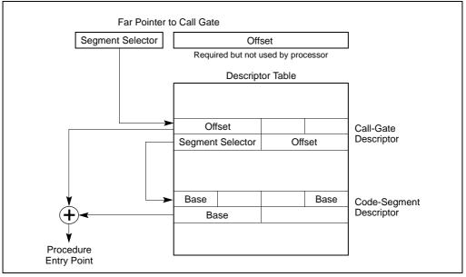
Figure 4-10. Call-Gate Mechanism
