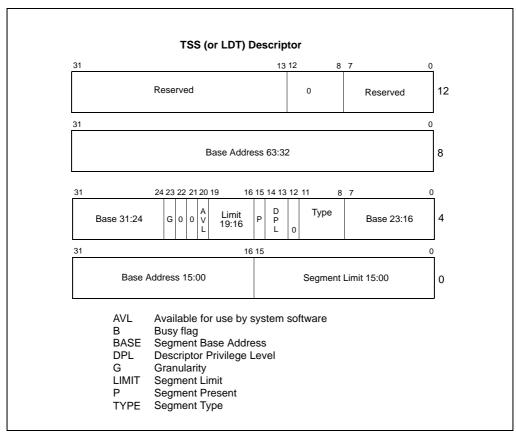
Figure 6-4. Format of TSS and LDT Descriptors in 64-bit Mode
