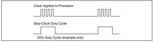
Figure 13-3. Processor Modulation Through Stop-Clock Mechanism
