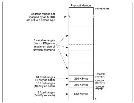
Figure 10-3. Mapping Physical Memory With MTRRs
