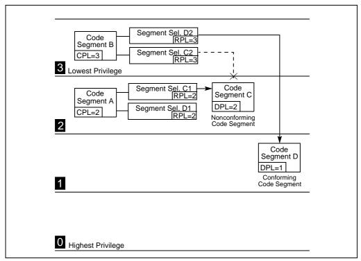
Figure 4-7. Examples of Accessing Conforming and Nonconforming Code Segments From Various Privilege Levels
