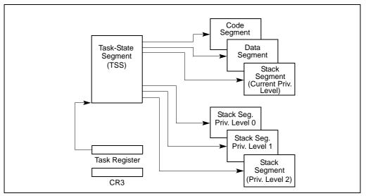
Figure 6-1. Structure of a Task
