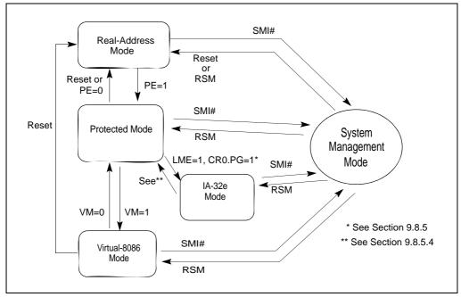
Figure 2-3 shows how the processor moves between operating modes.
