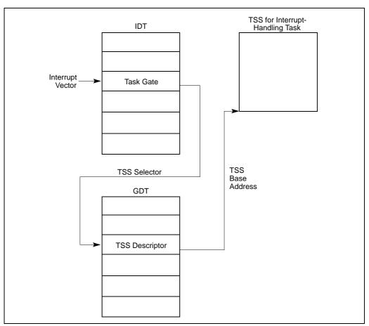
Figure 5-5. Interrupt Task Switch
