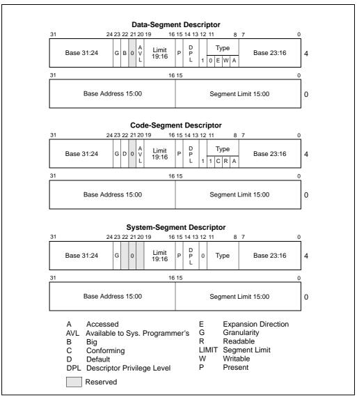
Figure 4-1. Descriptor Fields Used for Protection
