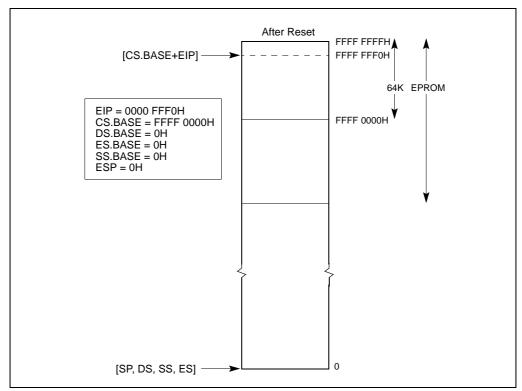
Figure 9-3. Processor State After Reset
