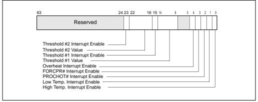
Figure 13-10. IA32\_THERM\_INTERRUPT Register
