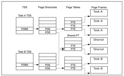
Figure 6-9. Overlapping Linear-to-Physical Mappings
