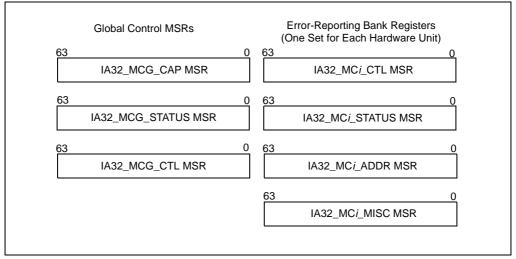
Figure 14-1. Machine-Check MSRs
