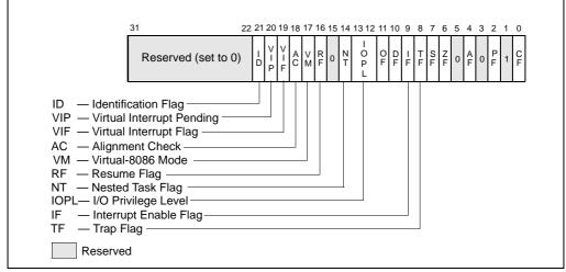
Figure 2-4. System Flags in the EFLAGS Register
