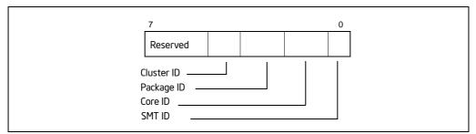
Figure 7-5. Generalized Four level Interpretation of the initial APIC ID
