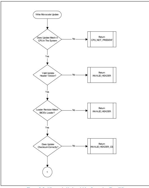
Figure 9-8. Microcode Update Write Operation Flow [1]
