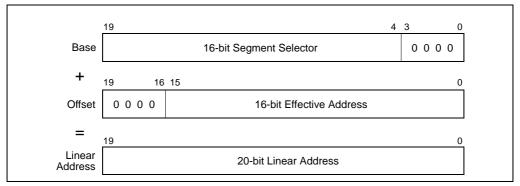
Figure 15-1. Real-Address Mode Address Translation
