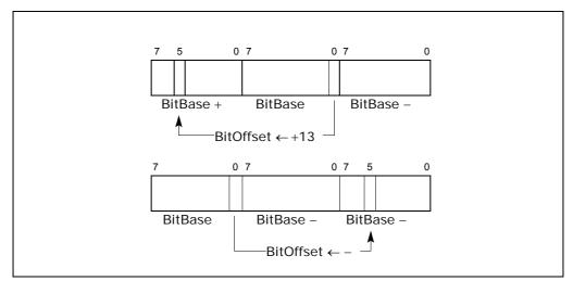
Figure 3-2. Memory Bit Indexing
