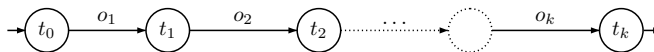
Figure 4.11. Observation sequence O = o_1 \cdots o_k . The time stamps t_i , i = 0, \dots, k , labeling states are multiples of 10 ms.
