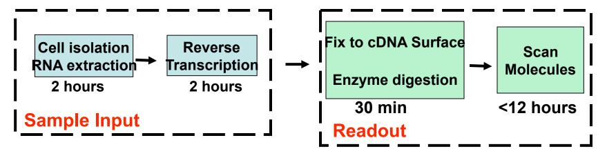
Microfluidic Device + Fast AFM
