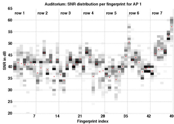
Figure 5. WiFi signal-to-noise ratio (SNR) distribution of the 49 fingerprints in the open-space environment (auditorium). Only access point AP 1 is shown here. Each vertical line corresponds to one fingerprint; the “higher” the count in the corresponding bin of the signal histogram. Each fingerprint was sampled at least 60 times, and the multimodal nature of the signal is apparent for some fingerprints.
