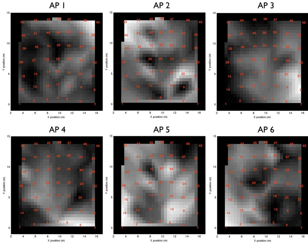
Figure 4. Mean values of the WiFi signal-to-noise ratio (SNR) interpolated every 0.5m between the 49 fingerprints in the open-space environment (auditorium). Signal “heat maps” from all 6 access points are shown.
