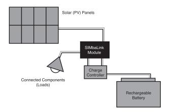
Fig. 1. A diagram of the integration of SIMbaLink with the other components of a solar home system.
