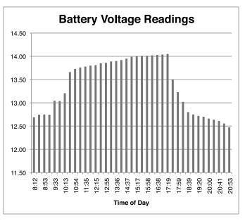
Fig. 4. These are sample voltage readings that were gathered from our test deployment in Figure 3. Voltages were measured on June 26.
