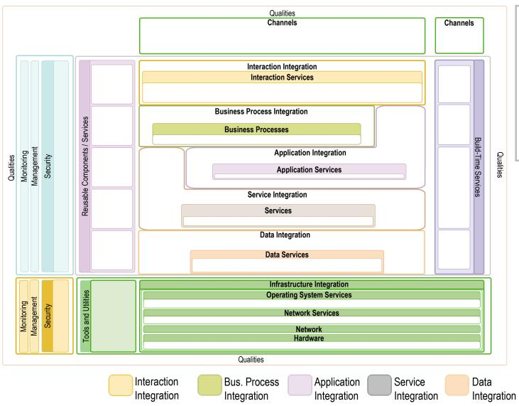
Separation of concerns through layering enables high cohesion and low coupling across the application components
