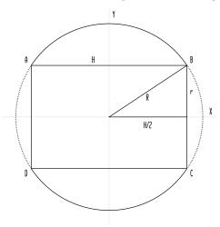
In this figure the rectangle with corners A, B, C, and D is the cross-section of the hole, and the segment above the chord A-B generates the portion of the sphere remaining. The volume remaining is
