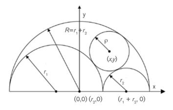
Place the centers of the three semicircles on the *x*-axis of a Cartesian coördinate system whose origin is at the center of the left semicircle. The figure above shows the radii and the coördinates of the centers of the three semicircles and the tangent circle.
