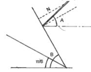
If *F* is the magnitude (force, momentum, or whatever) quantifying the impact strength, its component normal to the windshield with angle *B* (see the left figure below) is
