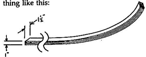
He wants to make a two-piece mold for gluing the strips together. He plans to cut an 8' sheet of plywood 1.5" thick, so the cut edges will be the surfaces of the mold.
