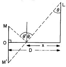
The image of M is located at M' and does not move at all (unless the floor is suddenly tilted!). The point K is the intersection of the line of sight L-M' with the floor. We "note from physics" that  $\theta = \theta'$ . Physics does not say anything about the relationship between 0, x, and D. That is high school geometry, as is the following statement: Two triangles having the same values for two of their angles are similar triangles. Hence:
