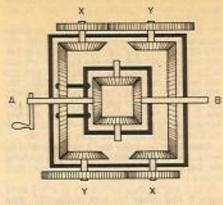
The back of the box has duplicate X and Y gears as on the front, but they are assembled as shown. All four inside bevel gears are duplicates. The two ring gears are duplicates, but the left one is riveted to the center differential gear box. Gearing locks boxes, so crank A drives shaft B in opposite rotation. If gears X and Y on the front are now interchanged, the differential gear box can rotate and shafts A and B can be turned independently, as required.
