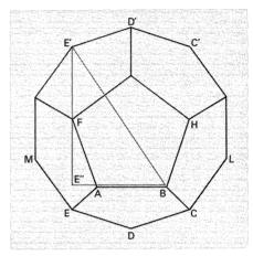
Thus the volume is 12 x 1/3 x area of one face x radius of the inscribed sphere (R). The last term is difficult. On the sketch, let E" be the projection of E' on the plane of the base ABC. Then  $(2R)^2 = (E'E'')^2 = (E'B)^2 - (E''B)^2$ . To obtain E'B, pass a plane through FHL, etc., and as the sides of the pentagon formed are diagonals of the faces, diagonals of this larger pentagon (e.g., MH) = e  $(3 + \sqrt{5})/2 = E'B$ . E"B = 2 x radius of circle inscribed in face
