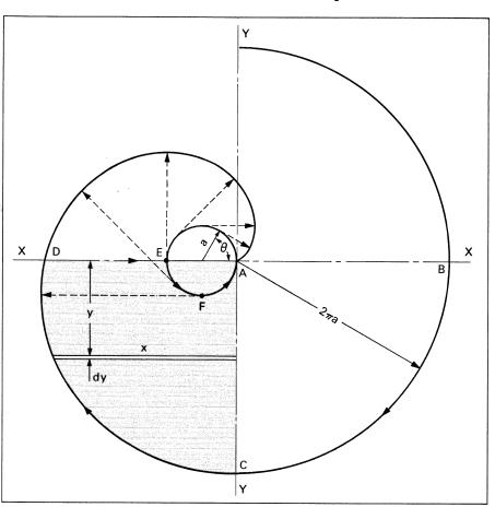
shaded in the drawing. The parametric equations of the involute of the circle with respect to the chosen coordinate system are
