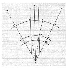
Bisect the given angle HXY with RX. Draw parallels AL and rO¹ at equal distances to RX. With X as center, swing arcs OS and dE. Bisect arc LS at I, and arc eE at M. Describe arc TP through O¹, where MI cuts the parallel. The angle is trisected at x and O¹, because MI is the locus of the midpoints of all the arcs drawn with X as center and contained between AL and XY. QEF and QED.
