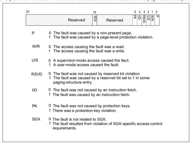
Figure 4-12. Page-Fault Error Code
