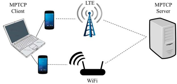
Figure 5: Setup of MPTCP measurement.
