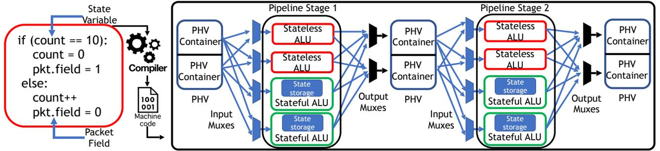
**Figure 1:** The left side shows a high level program (e.g., Domino, P4) given to the compiler. It is mapped to the Druzhiba RMT machine model on the right, which features a pipeline with depth and width of 2 and PHV length of 2. The pipeline stages' connections between PHVs to ALU inputs and ALU outputs to PHVs are also shown.
