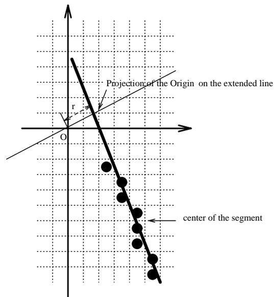
Figure 3.6: The thicker line is with parameter  $(\theta, r)$ . Projections of the pixels of this line onto line  $(\theta + 90^\circ, r)$  will disperse around the position  $r$  distant from the origin.
