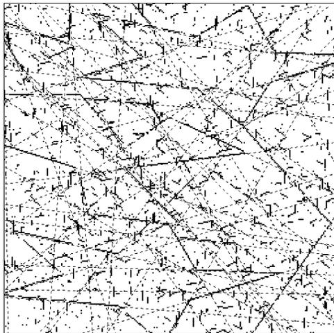
(c) 50 lines are detected using our improved Hough transform without proximity grouping.
