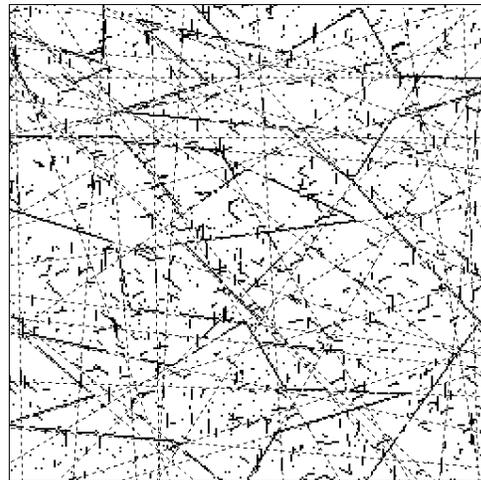
(d) 50 lines are detected using our improved Hough transform with proximity grouping.
