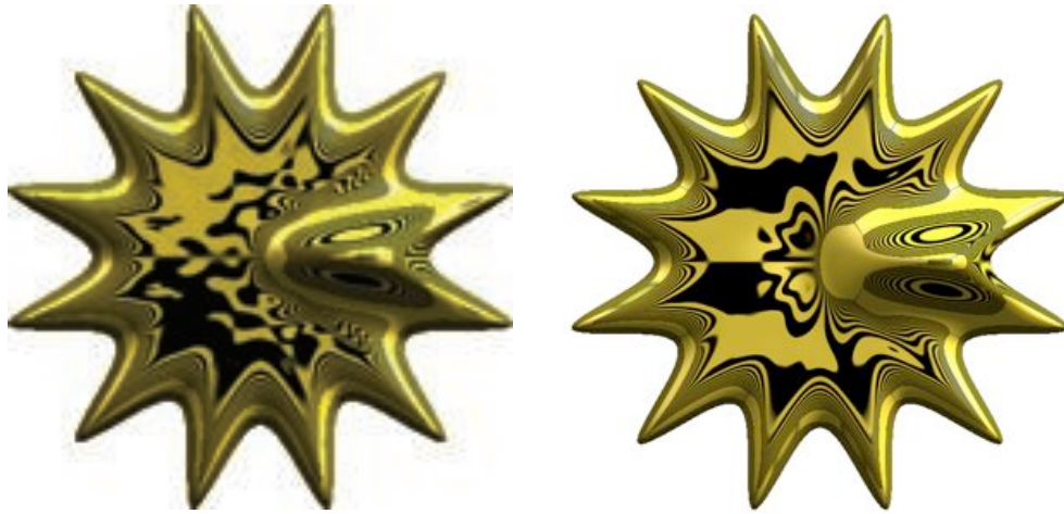
Figure 2.9: Left: A mesh with a valence 12 vertex fit using polynomials. Right: Same mesh fit using bi-cubic splines.
