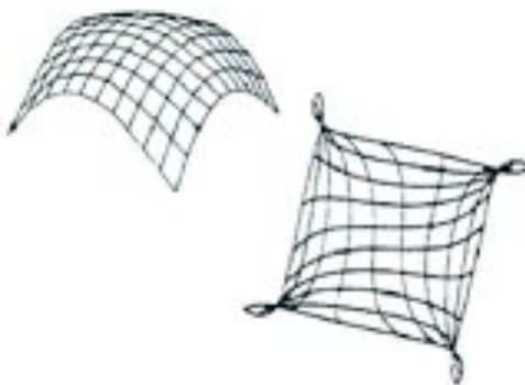
Figure 1.2: The orthotomic analysis of a bi-cubic patch [77].
