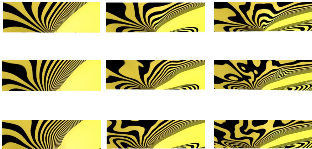
Figure 2.22: Top to bottom: Catmull-Clark, C^4 , C^\infty surfaces. Left to Right: Behavior near valance 3, valance 5, valance 7 boundary vertices.
