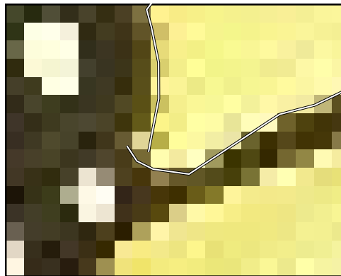
(a) Two separated edges can be joined, though some points should be removed to make a smoothed joining.
