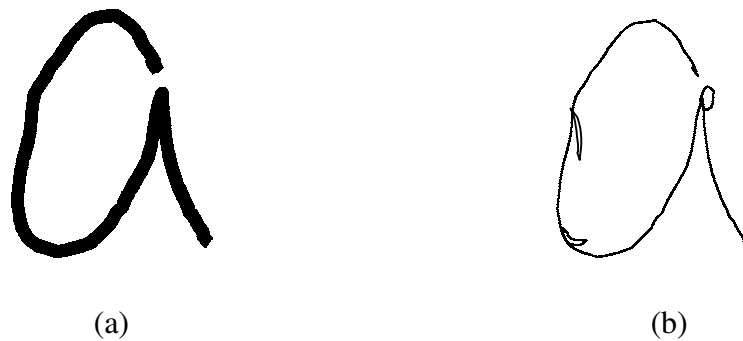
Figure 2. (a) Original off-line image (b) the result with some spurs after applying thresholding and thinning.
