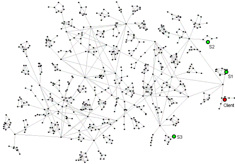
Figure 6.12: The 600-host network. The locations of the client and the three servers used in the experiment in Section 6.4.4 are shown.
