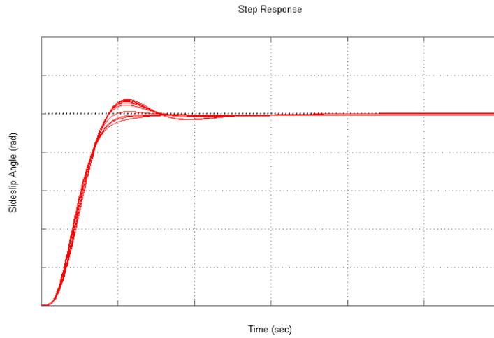
Figure 11: Integrated lateral  $H_\infty$  optimal CAS – Beta response.
