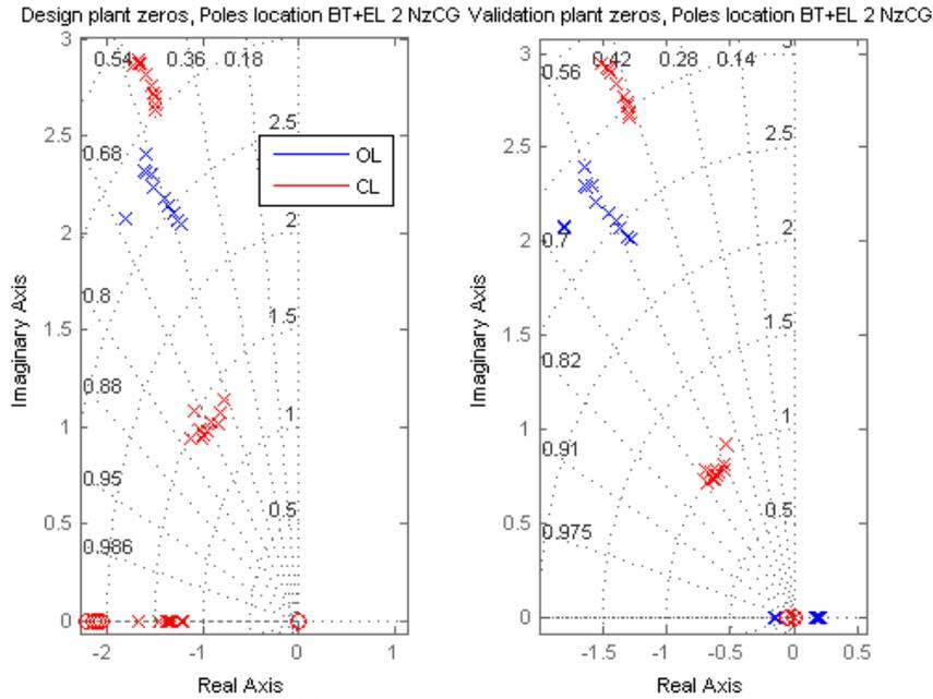
Figure 5: Poles and zeros location of BT+EL to Nz transfer function. All fuel cases are plotted for open loop (blue) and close loop (red).
