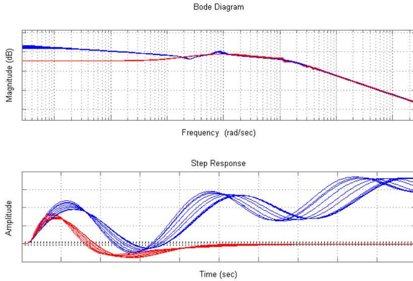
Figure 12: Dutch roll damper demonstration. Rudder to yaw rate step response and bode plot.
