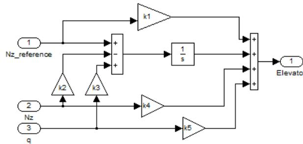
Figure 4: Longitudinal control law with structure.
