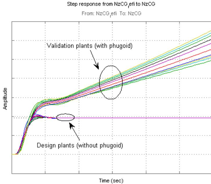
Figure 6: Nz reference signal tracking for all fuel cases. Design plant (without phugoid mode) and validation plant (with phugoid) are plotted. Axis description is hidden from confidential reasons for all next plots.
