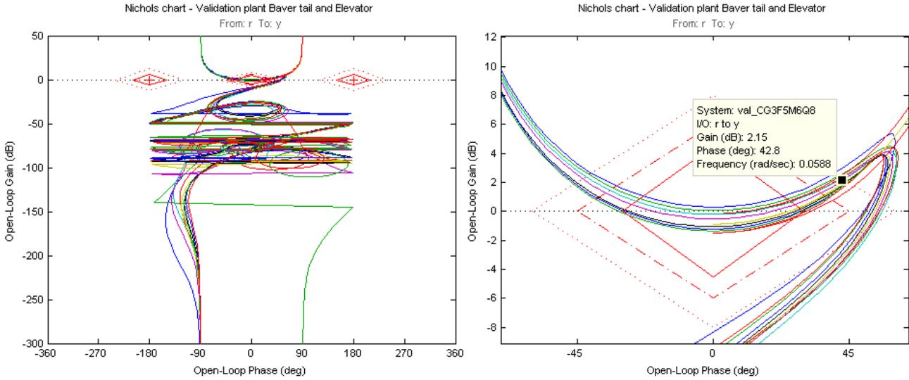
Figure 7: Nichol plots of closed loop (disconnected at control law output).
