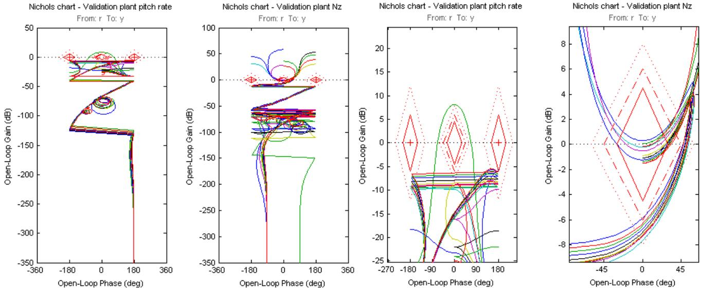
Figure 8: Nichol plots of closed loop (disconnected at control law inputs).
