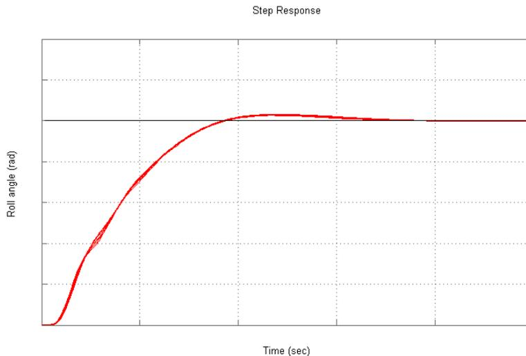
Figure 10: Integrated lateral H $\infty$  optimal CAS – Roll angle and rate response for all fuel cases.
