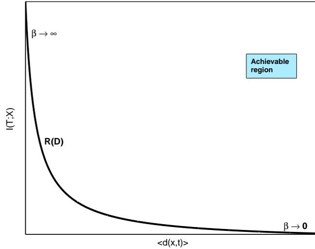
Figure 5: A typical rate-distortion curve, illustrating the trade-off between compression and average distortion. One can see that in order to achieve high compression (small  $I(T; X)$ ) a larger upper bound on the expected distortion must be used.
