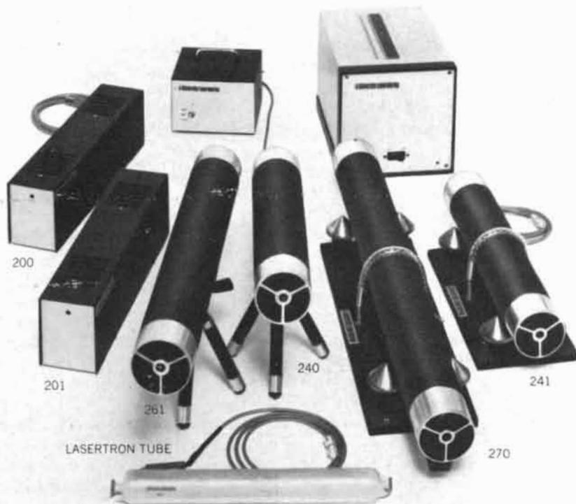
**The Lasertron® Tube** A coherent light bulb, it is the heart of every U/L laser. Never needs adjustment or maintenance. Simply switch it on or off. Resonator mirrors are permanently aligned inside a rigid pyrex envelope. Unaffected by dust, humidity, vibration, temperature or aging. Available as an OEM component or as part of complete instruments, as shown.
