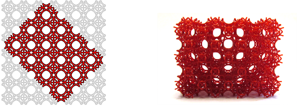
Figure 3.6: We extracted a 45^\circ rotated rectangular block from a regularly tiled 10mm cell microstructure to test Young’s modulus in non-axis aligned directions.
