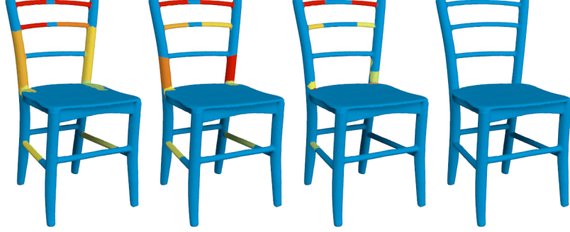
Figure 4.4: Weak regions extracted from three modes with weakness level cutoff, \epsilon = .10, .05, .01 .
