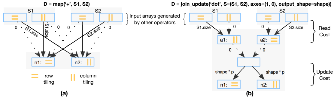
Figure 2.7: Two examples of building the tiling graph. (a) A plus expression, (S1 + S2) , implemented by map operator (b) A dot expression, dot(S1, S2) , implemented by join_update operator.
