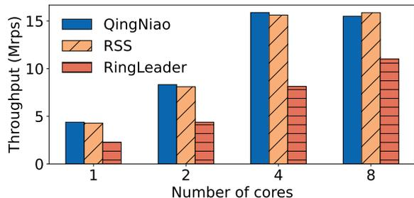
**Figure 4.15:** QingNiao achieves comparable performance as hardware L3/4 dispatcher.
