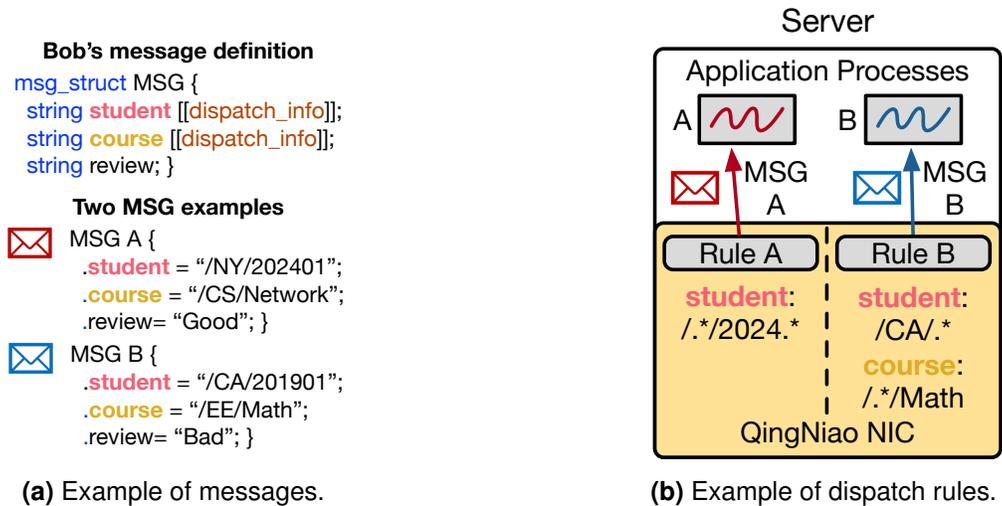
**Figure 4.3:** Example of the message struct definition and dispatch rules.
