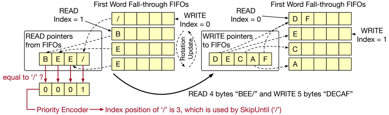
**Figure 4.7:** A BytePipe example with read and write index being 1 and 0 at the beginning, respectively. A *read* operation reads out 4 bytes (i.e., “BEE/”) and a following *write* operation writes in 5 bytes (i.e., “DECAF”). BytePipe leverages a priority encoder to indicate the position of the specified character used by SkipUntil(‘/’).
