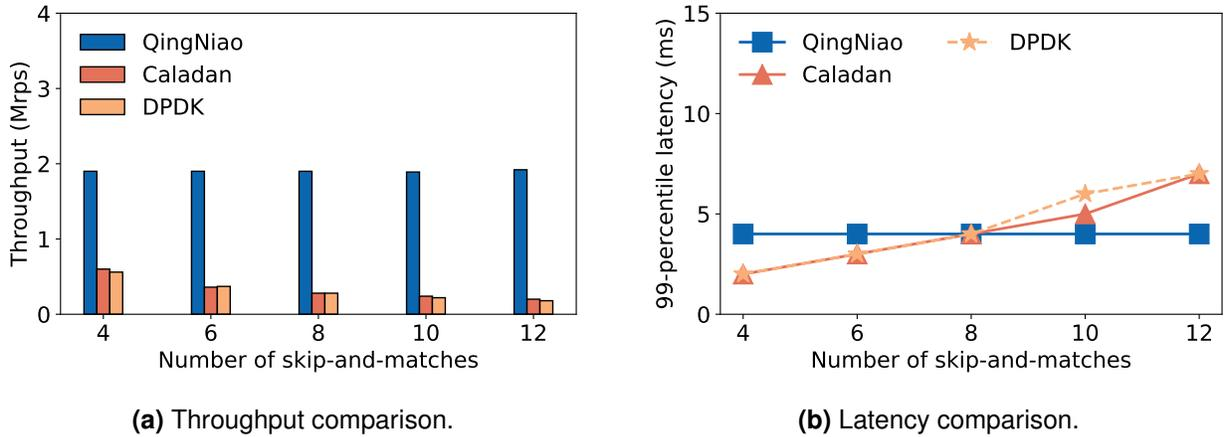
**Figure 4.11:** On throughput, QingNiao outperforms Caladan by 6.54× averagely with varying the number of skip-and-matches.
