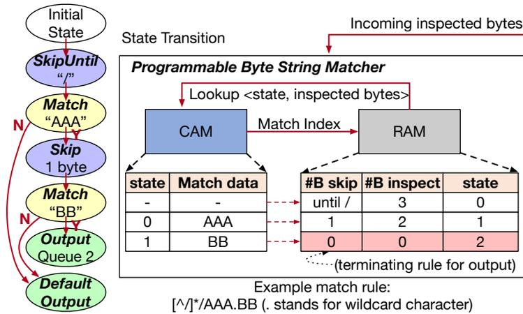
**Figure 4.8:** Matcher implements the skip-and-match. Skip and Match are encoded in RAM and CAM entries respectively. RAM entries with skipping and matching 0 bytes denote exit states: it shows the output queue index in the last column.
