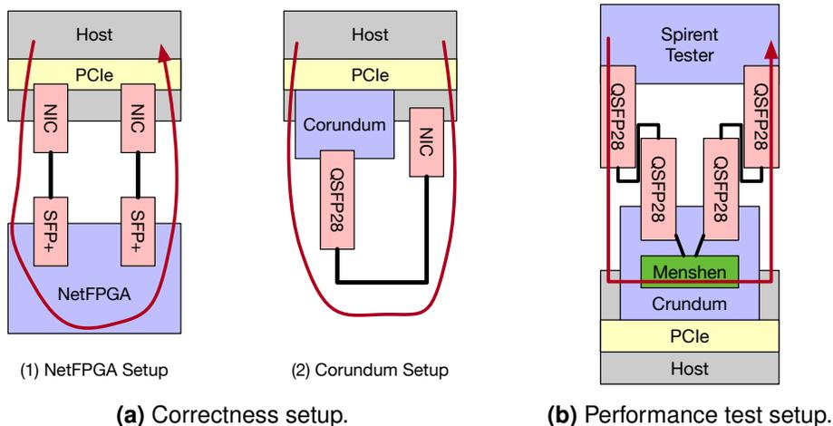
**Figure 3.8:** Testbed setup. Red arrow shows packet flow.
