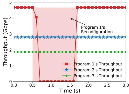
**Figure 3.12:** Disruption-free reconfiguration measured every 0.1 s.
