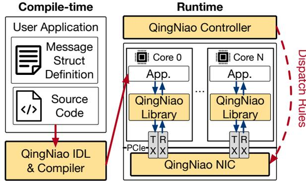
**Figure 4.2:** QingNiao’s design consists of the colored components.
