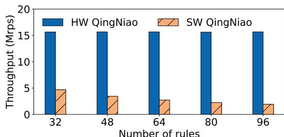
**Figure 4.17:** QingNiao outperforms software implementation by 5.74× averagely with varying number of rules.
