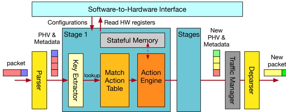
**Figure 2.1:** Example of an RMT pipeline.
