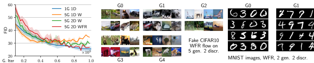
Figure 2.3: Training mixtures of GANs over CIFAR10. We compare the algorithm that updates the mixture weights and parameters (WFR-DA flow) with the algorithm that only updates parameters (W-DA flow). Using several discriminators and a WFR-DA flow brings more stable convergence. Each generator tends to specialize in a type of images. Errors bars show variance across 5 runs.
