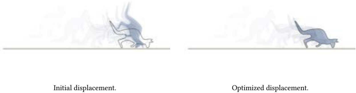
Figure 3.17: Non-linear transient simulation of a kangaroo (blue surface) bouncing on a plane to match a target shape (wire-frame).
