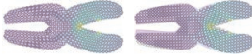
Figure 4.21: Left: deformation result after one level of quad mesh refinement when using our new method. Right: result using regular grid with cut cells.
