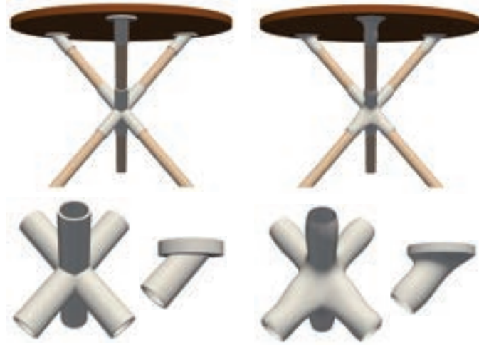
Figure 2.24: Left: the initial stool model; Right: the result after optimizing the white (PLA) pieces.
