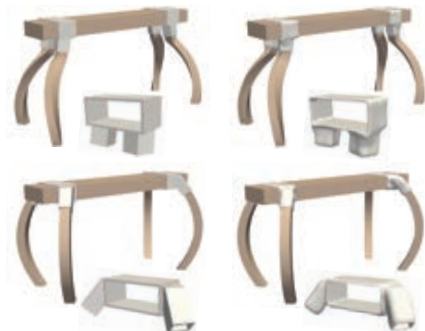
Figure 2.26: Bench model with two different types of legs and the initial and optimized connectors.
