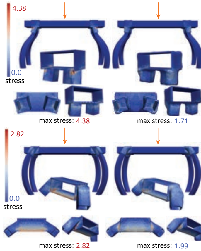
Figure 2.27: Bench stress for twisted and bended set of legs
