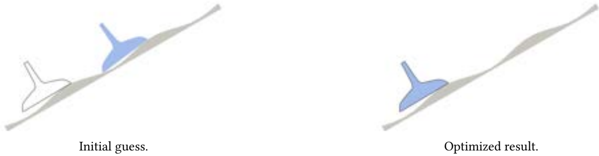
Figure 3.18: Optimization of the friction (blue surface) to match the target shape (wire-frame).
