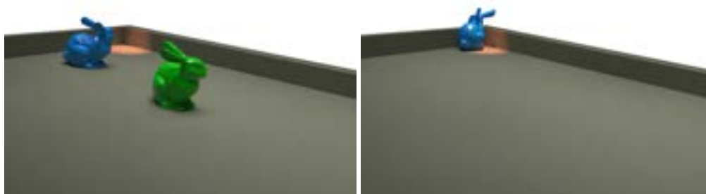
Figure 3.12: The initial conditions of the green bunny (left) are optimized to push the blue bunny in the corner of the pool table (right).
