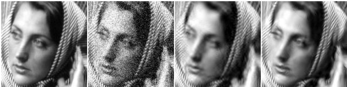
Fig. 6. Comparison of denoising results on Barbara image (cropped to 150 \times 150 for visibility of the artifacts). Left to right: Original image; Noisy image ( \sigma = 25 , PSNR = 20.2dB); Results of Li et al. [30] (PSNR = 28.2dB); Our method (PSNR = 29.1dB).
