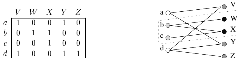
Figure 14: The matrix on the left is the input to the 2-populations problem. The corresponding bipartite graph for the Cut Classification (CC) problem, which is a min-cut problem, is as shown. The min-cut is of size 0 with the partitions \{b, c, W, X\} and \{a, d, V, Y, Z\} . Thus the 2 populations are \{a, d\} and \{b, c\} and the cut classifications are \{V, Y, Z\} and \{W, X\} .
