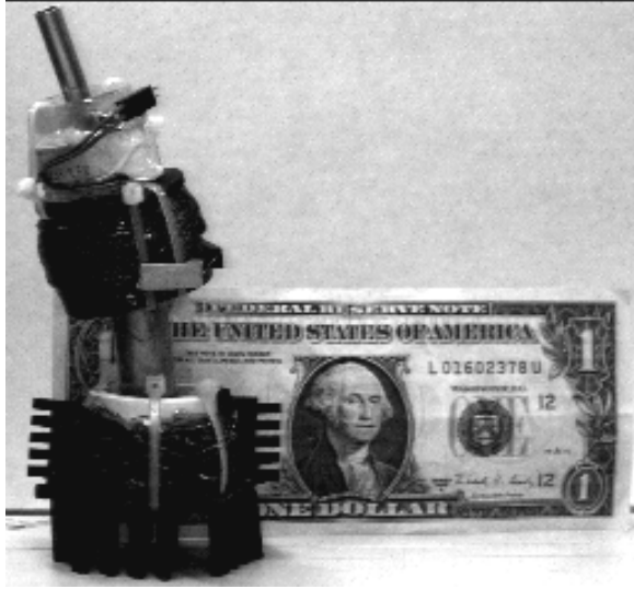
Figure 3: The direct drive finger is a three link mechanism made of stacked coil and magnet pairs. Maximum force at the fingertip is 1.0 Nt, and fingertip force is determined by controlled torques at the joints. The finger has no gears and therefore has passive dynamics.
