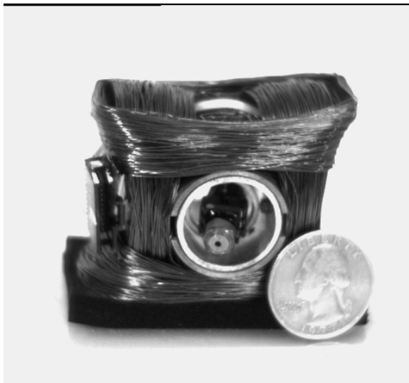
Figure 3: The Spherical Pointing Motor and camera sensor. The camera head (CCD and lens assembly) measures only 8 \times 8 \times 10 mm. The SPM takes up a volume 4 \times 5 \times 6 cm.
